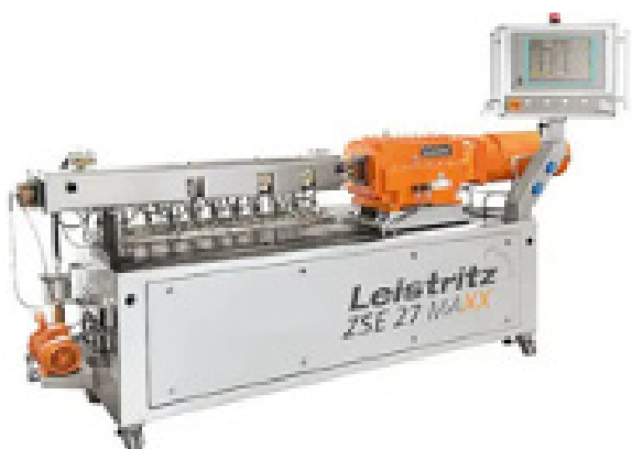
Figure 4. Leistritz ZSE 27MAXX compounding line.
