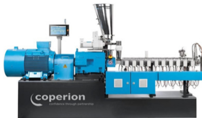
Figure 2: Reactive extrusion Pilot Line available at AITEX facilities
